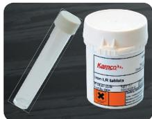
Mains water often contains iron, although at levels of less than 1 mg/l. A test reading of more than 1 mg/l above the mains water indicates that corrosion is taking place (even though water drawn from the top of a radiator may be clear), and the system should be power flushed.
